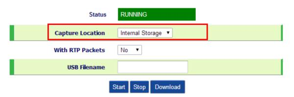
Figure 9: Capture to Internal Storage
