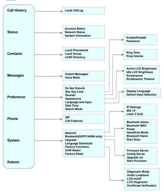
Figure 1: Keypad MENU Configuration
