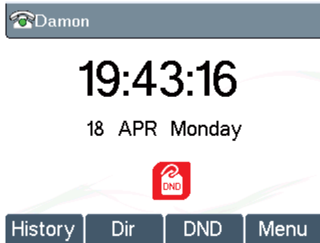
Figure 46 - DND Enabled on All Lines
