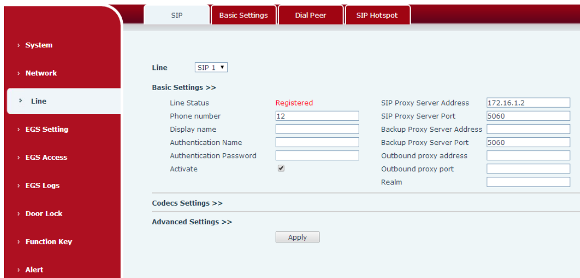
Figure 4 - SIP Line Configuration
